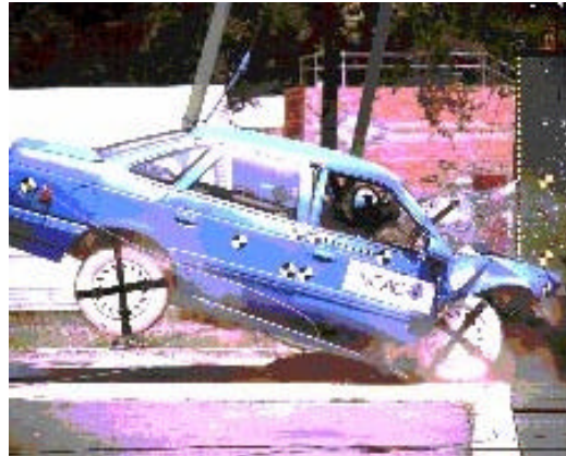
The NCAC conducts a 50-mph crash test to validate a computer model of the Ford Taurus.
